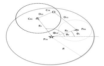
Figure 2: System model layout of cognitive radio adhoc network using spectrum of primary spectrum.
