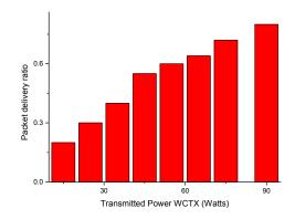
Figure 9: Data transfer in packets when C<sub>RX</sub> moving at average speed 45m/s
