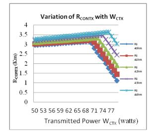
Figure 4: Power transmitted vs. concurrent transmission radius
